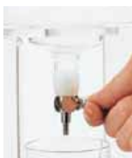
Use the faucet to adjust dripping rate.
